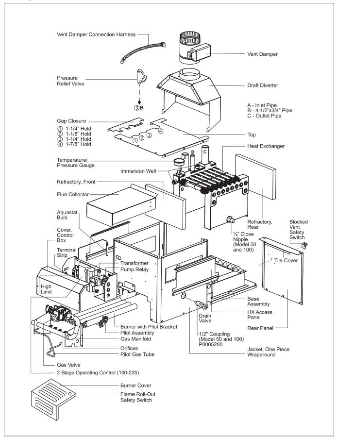
Figure 15. Parts Identification.
